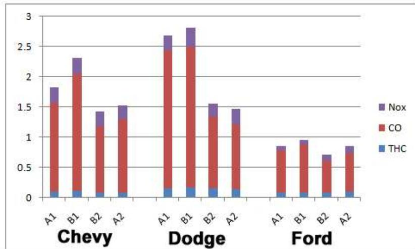
**Graph 3** Regulated toxic emissions trends from stock (A<sub>1</sub>), immediate installation (B<sub>1</sub>), after mileage accumulation (B<sub>2</sub>), and back to stock again (A<sub>2</sub>).
